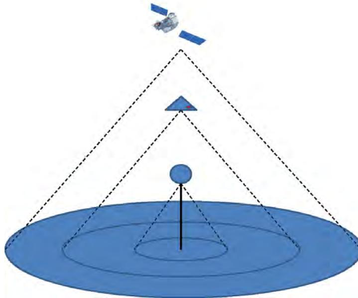
Fig.5 The fastest possible detection would depend on the SAoI size and the altitude of the surveillance asset assuming the same sensor field-of-view and that spatial resolution on the ground is not compromised as the area of sensor coverage is increased.
