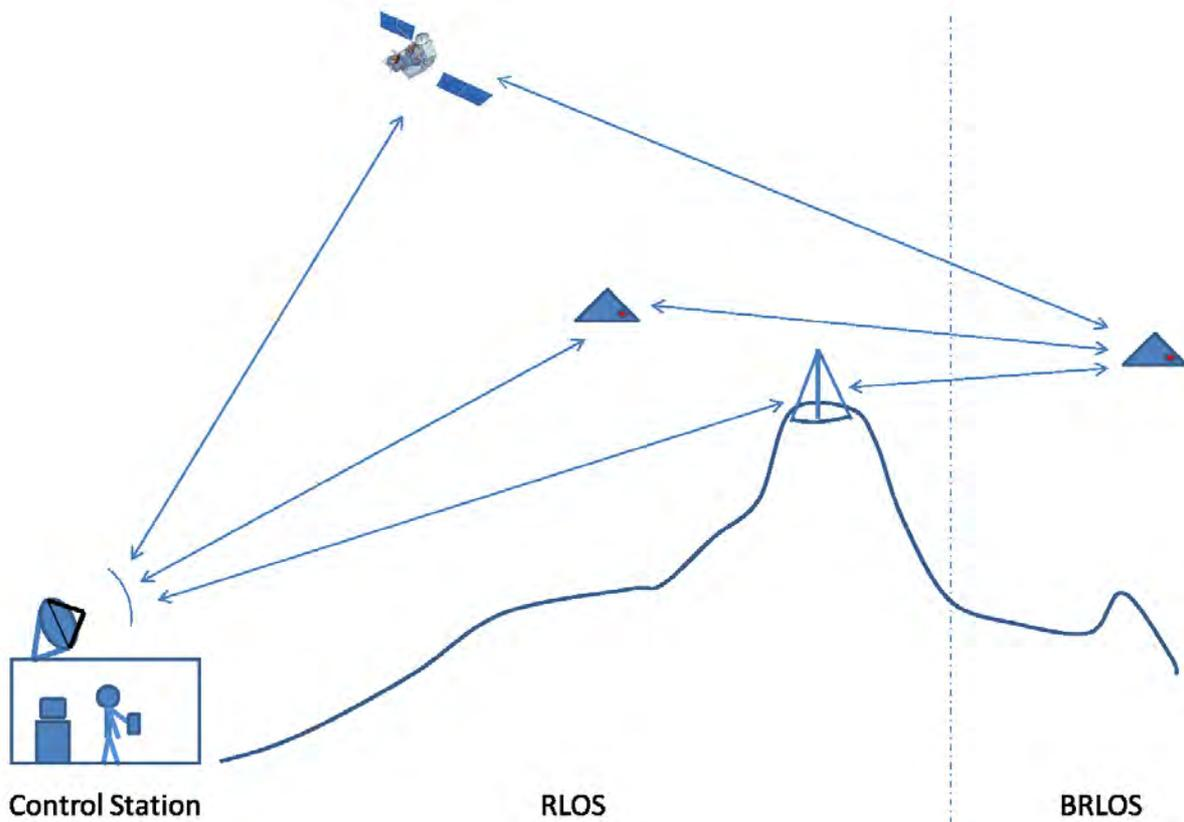
Fig.13 Use of multiple assets for enabling Beyond Radio Line of Sight communications between the RPA and the control station.
