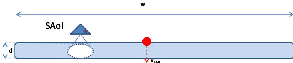
Fig.6 A simplified case having 100% detection probability where the SAoI is confined in a straight line with dimensions  $w$  and  $d$  (equal also to the diameter of sensor coverage of the RPA). A target will be detected if stationed within the SAoI or if travelling at a speed which does not allow it to travel the distance  $d$  of the SAoI faster than the RPA can scan the whole SAoI ( $V_{TAR} \leq V_m \cdot d/w$ ).
