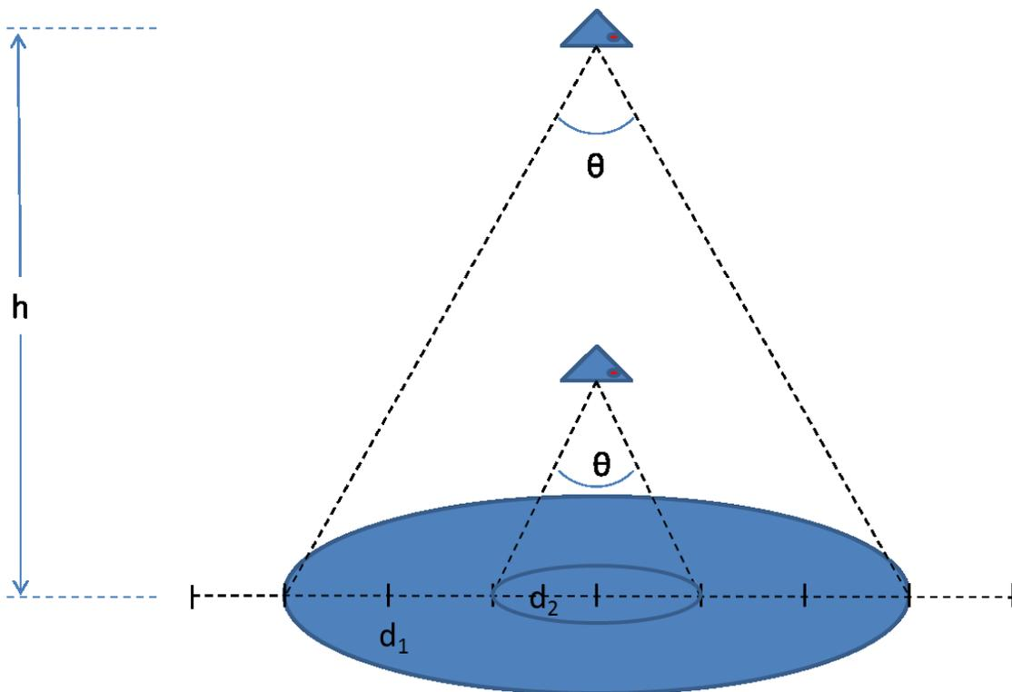
Fig.8 The figure shows that if the RPAS altitude ( $h$ ) is increased while the field of the view and spatial resolution of the sensor at the ground remain the same (or adequate) then the diameter of the area of sensor coverage  $d$  increases thus reducing mobility requirements for the RPAS (vertical view case).
