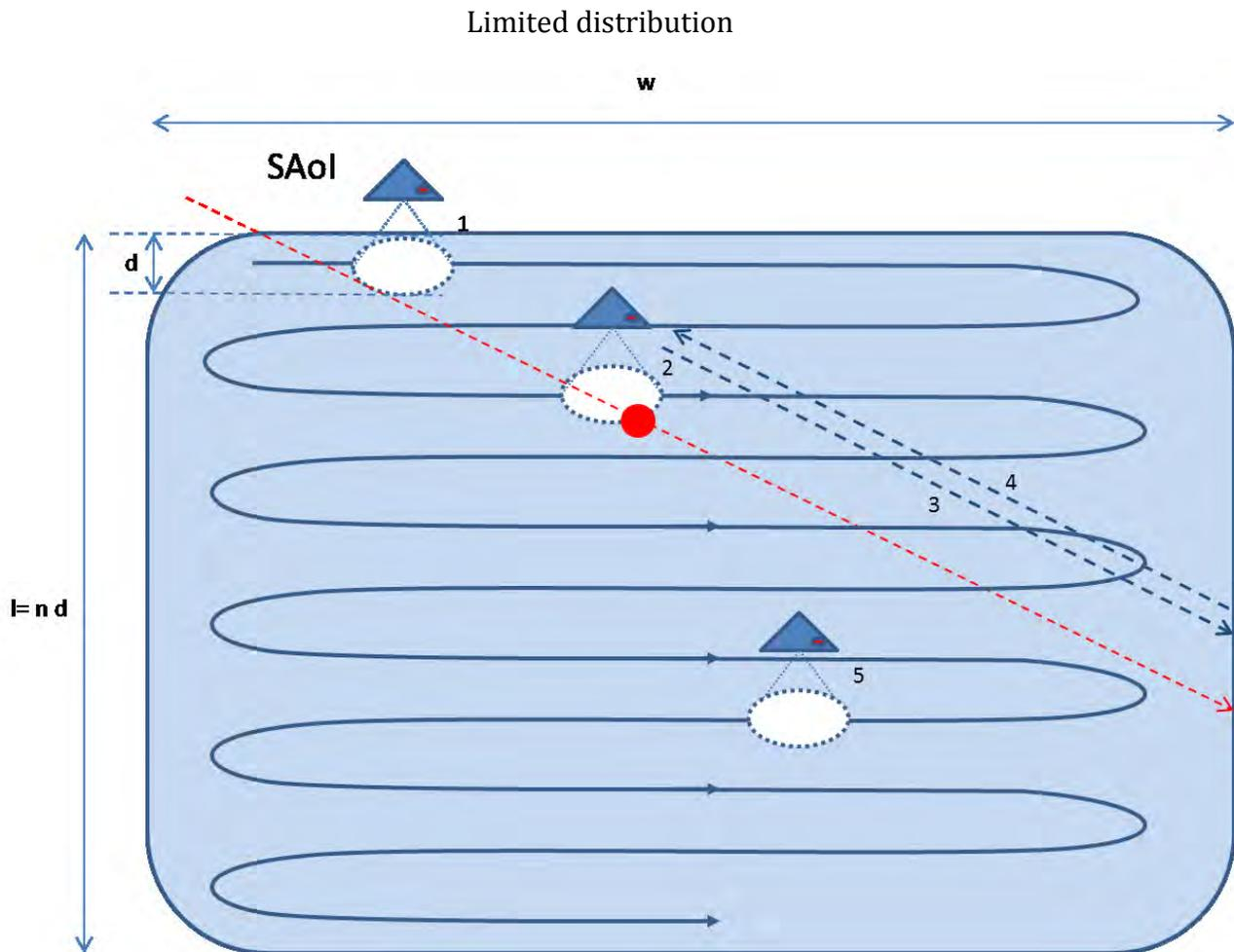
Fig.7 A diagrammatic representation of a possible operational concept of a mission including detection, classification, identification and tracking of targets of interest within a SAoI.
