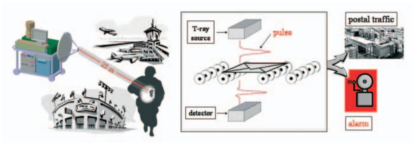
TERAHERTZ SCANNER FOR STAND-OFF DETECTION AND LETTER INSPECTION
