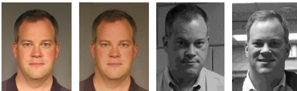
Figure 3: From left to right: original reference; reference printed, scanned (300 dpi), resized (360x465 pixels) and compressed (JPEG 2000, 15KB); probe with slight rotation; probe with changing expression and variation in illumination.
