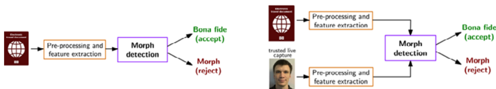
Figure 1: Morphing attack detection scenarios. Left: Single image Morphing Attack Detection, Right: Differential Morphing Attack Detection
