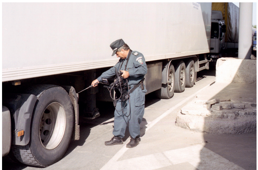
Figure 2. A Hungarian police officer sets a sensor of a heart beat detector and a flexible camera to search for irregular migrants during control of a lorry at the border between Hungary and Serbia near Rösztke
