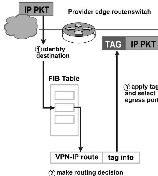
MPLS is an IETF standard technology that speeds up network traffic flow by avoiding packet analysis by intermediate routers (hops). This is done on the basis of so-called labels that are attached to packet by the edge routers of the backbone, on the basis of information stored in the forwarding information base (FIB). Labels are also used to implement virtual private networks (VPNs).
