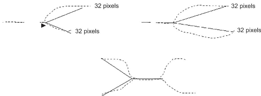
The angle of the minutiae is determined by constructing three virtual rays originating at the bifurcation point and extending to the end of each leg. The smallest of the three angles formed by the rays is bisected to indicate the minutiae direction.
