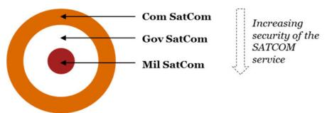
**1 MILSATCOM:** MILSATCOM is highly protected and guaranteed SATCOM, generally provided by military systems, offering highly assured and protected satellite communication capacity both in terms of nuclear hardening, anti-jamming/dazzle
