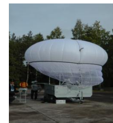
AERONAUTICS SKYSTAR 180 Tactical aerostat All weather conditions
